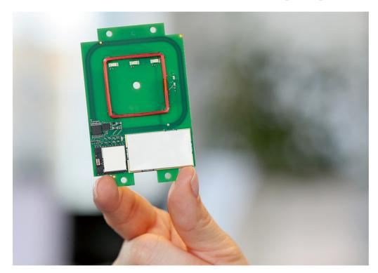
The TWN4 MultiTech 2 family of contactless RFID readers and modules from ELATEC enables users to read and write to almost any RFID standards-compliant low- and high-frequency tags and labels. They also support NFC connectivity.
