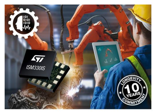
The ISM330IS motion sensor from STMicroelectronics, which combines a three-axis digital accelerometer and a three-axis digital gyroscope, contains a processing unit to provide real-time sensor data to the host application.
